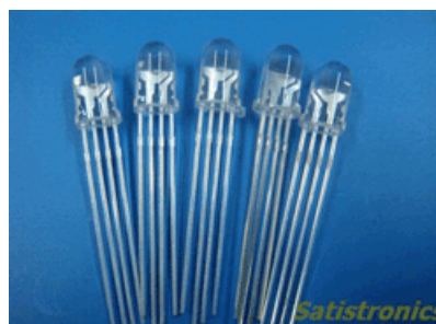
Figure 6: Red, green, blue (RGB) LEDs
